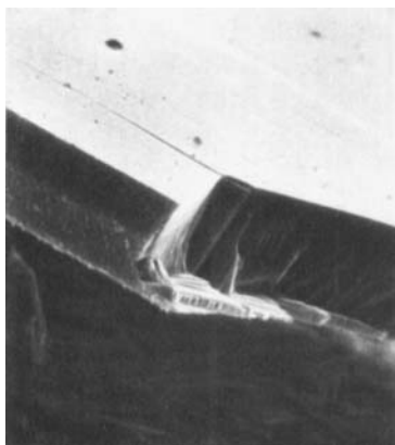
A fractured end of (\text{TMTSF})_2\text{ClO}_4 magnified 500 times
